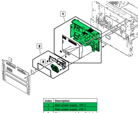
2 Main power supply fan with duct 3 Main power supply fan
