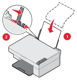
2 Squeeze the release tab, and slide the paper guide to the right until it rests against the edge of the paper.
