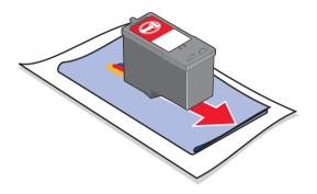
4 Using another clean section of the cloth, gently hold the cloth against the contacts for about three seconds, and then wipe in the direction shown.
