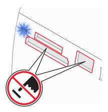
If the printer does not read the memory card, remove and reinsert it.
