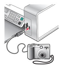
The message PictBridge camera detected. Press ① to change settings. appears on the display.
