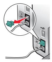
**4** Connect a second telephone cord from the computer modem to the EXT port of the printer.
