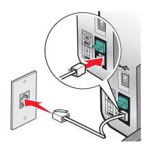
**3** Remove the protective plug from the EXT port of the printer.
