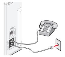
**Warning—Potential Damage:** Do not touch cables or the printer in the area shown while actively sending or receiving a fax.
