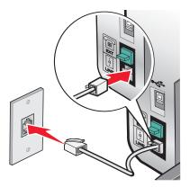
**3** Remove the protective plug from the EXT port of the printer.
