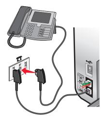
**5** If you would like to use the same line for recording messages on your answering machine, connect a second telephone line (not provided) between the answering machine and the other N slot of the telephone wall jack.
