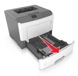
**2** Squeeze and then slide the width guide tab to the correct position for the size of the paper you are loading.
