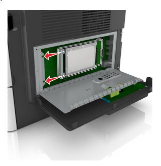
**c** Tighten the two screws.
