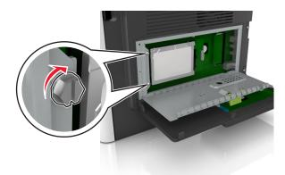
**d** Insert the plug of the printer hard disk interface cable into the receptacle of the controller board.
