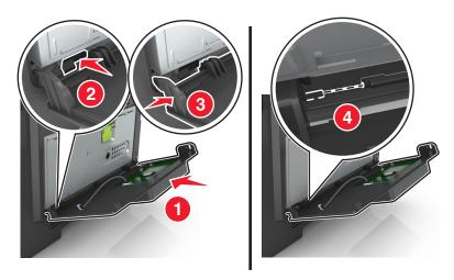
Run the ISP cable through the controller board shield door.
