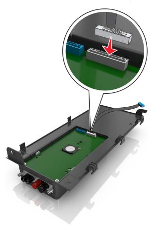
Slightly close the ISP exterior cover up to 65 degrees, and then slide the cover to attach.
