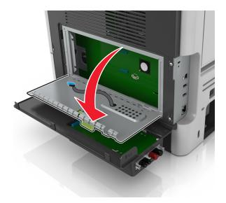
**12** Attach the blue plug of the ISP solution interface cable into the blue receptacle on the controller board.
