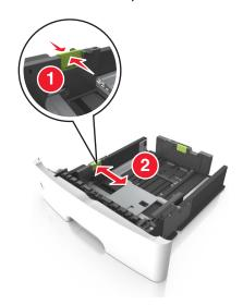
3 Squeeze and then slide the length guide tab to the correct position for the size of the paper you are loading.
