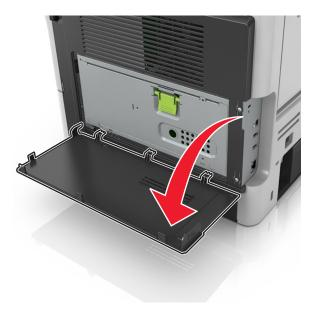
2 Lightly press the stop on the left side of the access door, and then slide the access door to remove.
