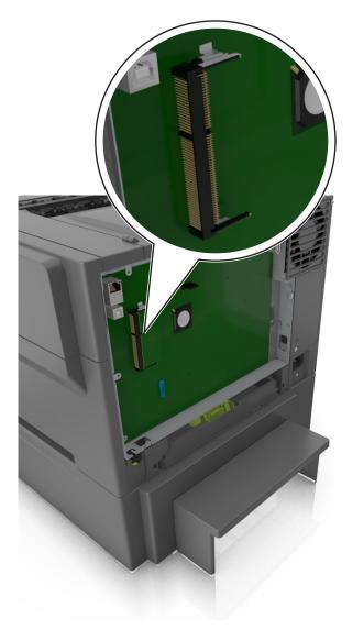
**Warning—Potential Damage:** Controller board electronic components are easily damaged by static electricity. Touch a metal surface on the printer before touching any controller board electronic components or connectors.
