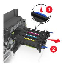
8 Remove the used developer unit.
