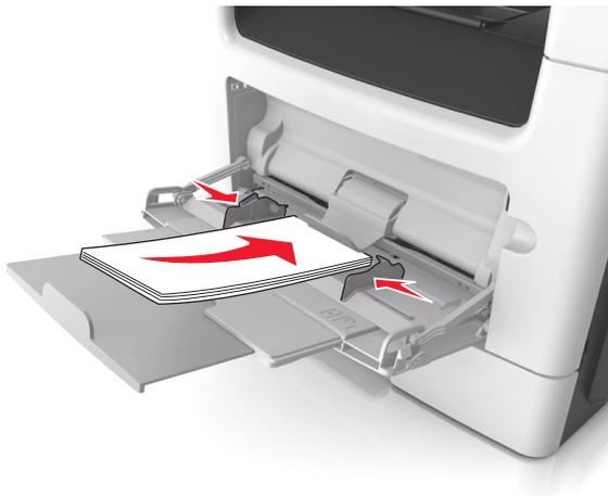
**Warning—Potential Damage:** Never use envelopes with stamps, clasps, snaps, windows, coated linings, or self-stick adhesives. These envelopes may severely damage the printer.
