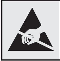
This symbol identifies static-sensitive parts. Do not touch in the areas near these symbols without first touching the metal frame of the printer.
