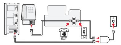
A Digital Subscriber Line splits your regular telephone line into two channels: voice and Internet. Telephone and fax signals travel through the voice channel, and Internet signals pass through the other channel. This way, you can use the same line for analog voice calls (including faxes) and digital Internet access.
