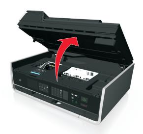
**Note:** The printhead moves to the cartridge installation position.
