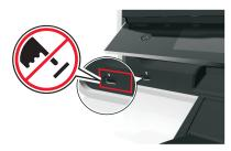
**Warning—Potential Damage:** Do not touch any cables, any network adapter, any connector, the memory device, or the printer in the areas shown while actively printing, reading, or writing from the memory device. A loss of data can occur.
