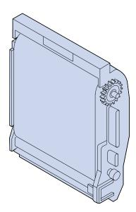
The photo developer cartridge receives toner from the toner cartridges. The toner image is generated on the photo developer media. The photo developer transfers the generated image onto the transfer drum so it can be placed on the print media you selected.
