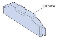
The oil bottle provides oil that lubricates the fuser. The approximate yield of the oil bottle is 12,000 pages. The average yield is determined by the number of printing of A4 or letter size pages printed.
