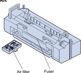
The fuser uses heat and pressure to permanently bond the toner to the print media. The air filter removes dust and other contaminants from the printer. You receive a new filter each time you order the fuser kit. The approximate yield of the fuser and air filter is 40,000 pages.
