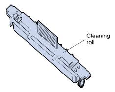
The cleaning roll removes excess toner and other contaminants from the fuser. It is located under the top door. The approximate yield of the cleaning roll is 12,000 pages. The actual yield depends on the toner coverage on each printed page.
