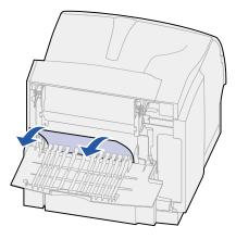
If the paper does not move immediately when you pull, stop pulling. Remove the print cartridge, and then pull the paper out.
