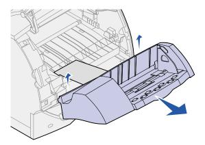
7 Pull the envelope straight out of the printer.
