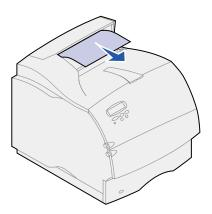
If the paper does not move immediately when you pull, stop pulling. Open the upper front door and pull the paper out.
