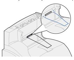
4 Carefully lift the option straight up until it is completely disconnected from the option below it or from the printer. Set it aside.
