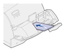
**Note:** Do not try to load more envelopes by forcing them under the envelope feeder weight. This results in jams.
