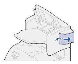
**2** Firmly pull the colored tab to remove the staple cartridge holder from the stapler.
