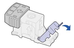
8 Push the cartridge holder firmly into the stapler until the cartridge holder *clicks* into place.
