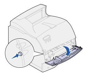
2 Locate the metal bar in the recessed area on the multipurpose feeder. Pull the bar out far enough to accommodate the paper you will be using.
