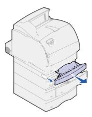
3 Pull the integrated tray out of the printer.
