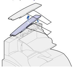
You must attach the top cover to the printer or topmost output option when you finish removing output options. In addition, it may be necessary to remove the paper bail from the top cover, depending on the type of output option to which it is attached. Refer to the *Setup Guide* for more information.
