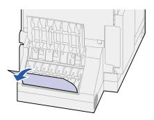
4 Pull down and out if the paper is in this position:
