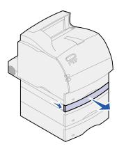
8 If the edge of the paper is visible, pull the paper straight up and out.
