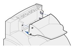
3 The output option may have a wire paper bail attached. If so, remove the tips of the paper bail from the ends of the plastic bracket on the bottom of the output option.
