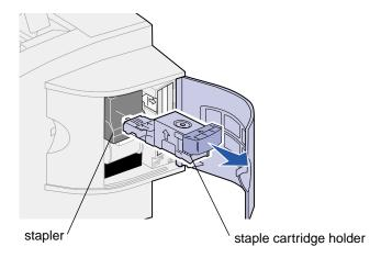
**3** Turn the cartridge holder as shown in the illustration in step 4.
