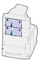
**Note:** If the jam occurs in a high-capacity output stacker, it may be necessary to open *both* of its rear doors.
