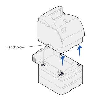
2 Carefully lift the option straight up until it is completely disconnected from the option below it. Set it aside.
