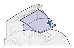
**b** Pull the tray straight out toward you to remove the upper tabs from the output expander slots.
