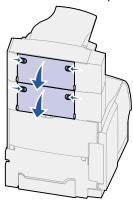
**Note:** Open *both* rear doors if the jam occurs in a high-capacity output stacker.
