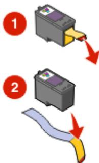
**Warning:** Do *not* touch the gold contact area on the back or the metal nozzles on the bottom of the cartridge.
