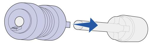
**b** Pull the pick roller gently to see if it is attached. If it pulls loose, then push it back on and turn it clockwise.
