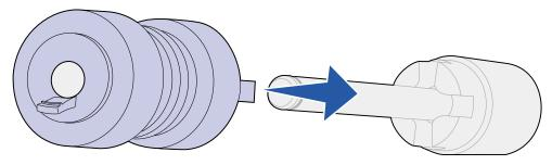
**12** Pull the pick roller gently to see if it is attached. If it pulls loose, then push it back on and turn it counterclockwise.
