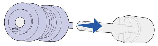
**7** Pull the pick roller gently to see if it is attached. If it pulls loose, then push it back on and turn it counterclockwise.
