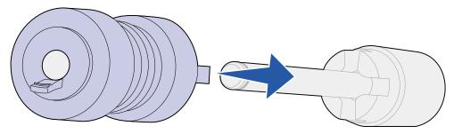
**b** Pull the pick roller gently to see if it is attached. If it pulls loose, then push it back on and turn it clockwise.
