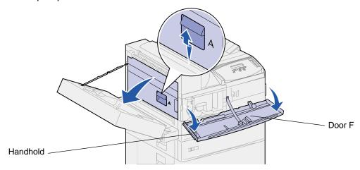
5 Using the handholds located on each side, pull open the printer front door (Door F).
