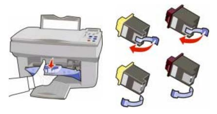
Place the cartridges into the carrier. Push back on the cartridges until they **snap** into place.
