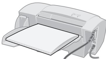
d Insert the leading edge of the first page into the sheet feeder.
