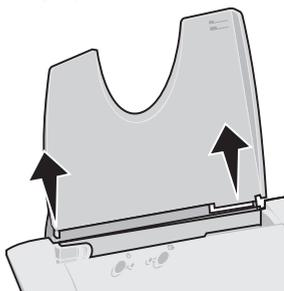
b Tilt the paper support back until it locks in the horizontal position.
