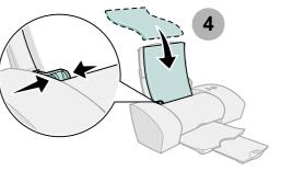
**Note:** A4 size paper should extend slightly above the top of the paper support. Letter size paper should align with the top of the paper support. Setup
