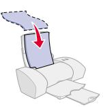
**3** Squeeze the release tab and the paper guide together. Slide the paper guide to the left edge of the paper
