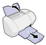
**2** Load up to 100 sheets of plain inkjet paper, and then squeeze and slide the paper guide to the left edge of the paper.
