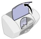
**Note:** The cartridge carrier moves to the loading position.
