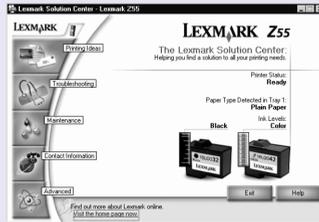
The Lexmark Solution Center is your complete guide to troubleshooting, cartridge alignment and maintenance, printing a test page, and the advanced features of your printer such as the paper type sensor.
