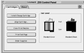
The Lexmark Z55 Control Panel or the Lexmark Z55 Utility is your complete guide to cartridge alignment and maintenance, printing a test page, obtaining information about your printer, and ordering supplies.
