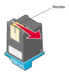
**d** Using another clean section of the cloth, gently hold the cloth against the contacts for about three seconds, and then wipe in the direction shown.
