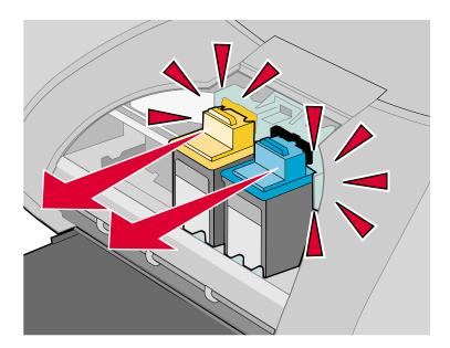
4 Remove the used cartridges. Store them in an airtight container or dispose of them properly. When removing the photo cartridge to exchange it with a black cartridge, store the photo cartridge in the storage unit provided.
