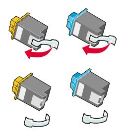
**Warning:** Do *not* touch or remove the gold contact area on the back and bottom of each print cartridge.
