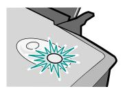
The print cartridge carrier is stalled.
