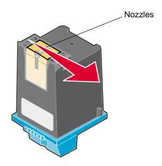
**d** Gently hold a clean section of the cloth against the contacts for about three seconds, and then wipe in the direction shown.
