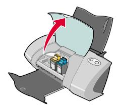
The cartridge carrier moves to the loading position, unless the printer is busy.
