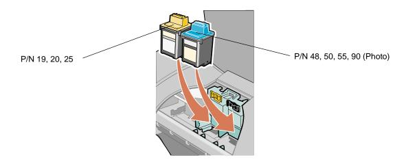
**Note:** To extend the life of your color cartridge and improve printing speed, install a black or photo cartridge along with the color cartridge.
