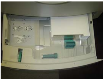
The Lexmark C920's 550-sheet universal trays accommodates paper weights up to 176 g/m2 (47 lb. bond) and has sliding guides on both axes.
