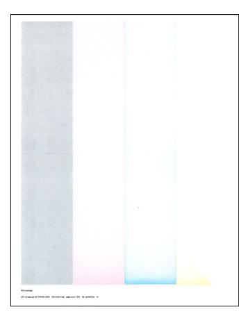
At meter count 622,027 impressions into testing on the CX860dte, BLI technicians replaced the Image Transfer Unit, which had reached end of life. Shortly thereafter, at meter count 641,623, BLI technicians noted that toner was not being properly transferred to pages. The page shown above should contain four solid bars of black, magenta, cyan and yellow. BLI technicians installed a replacement transfer unit and the issue was resolved.
