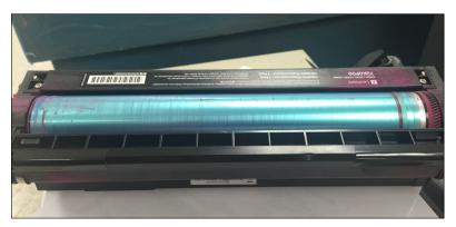
At meter count 799,128 impressions into testing, BLI technicians noted streaking on output. Upon further investigation, technicians noted that the magenta drum unit was defective. Replacing it with a new unit resolved the issue.
