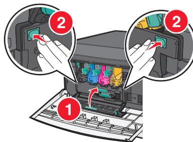
6 Insert the toner cartridge into the printer and then turn the toner lock lever to the left.
