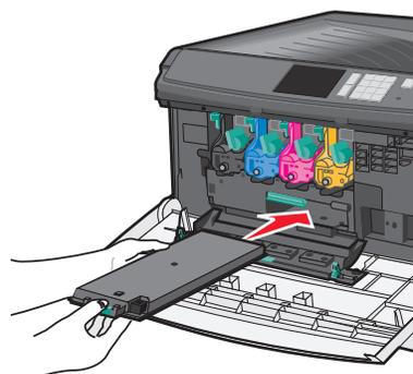
7 Using both hands, push the sides of the internal cover firmly until it *clicks* into place.
