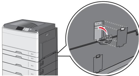
**8** Attach brackets to the back of the printer, optional tray, and printer stand.
