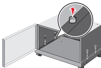
**b** Lift the upper portion of the printer stand, leaving the base.
