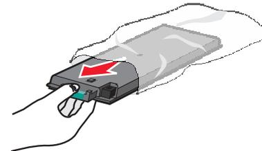
**6** Insert the new waste toner bottle into the printer.
