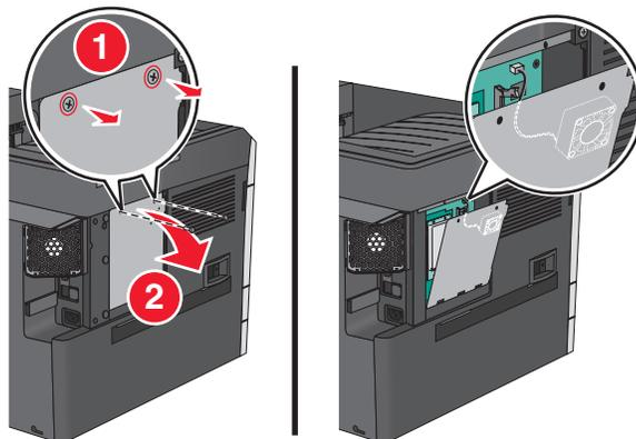
**Note:** Do not unplug the fan cable unless necessary.
