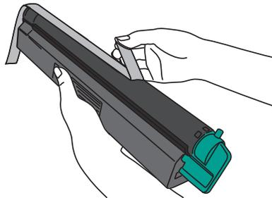
**10** Insert the toner cartridge and turn the lock lever to the left.
