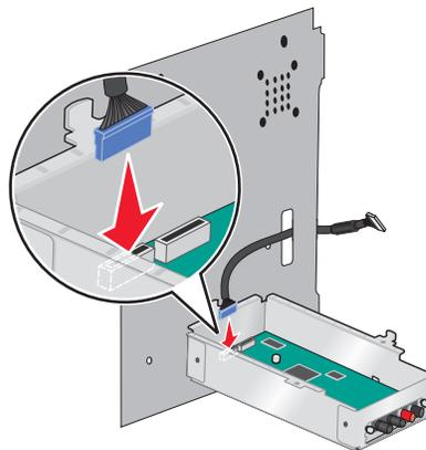
**11** Attach the ISP to the metal panel using three screws that came with the Connectivity Installation Kit.
