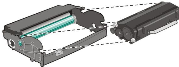
6 Install the unit into the printer by aligning the arrows on the guides of the unit with the arrows in the printer. Push the unit as far as it will go.
