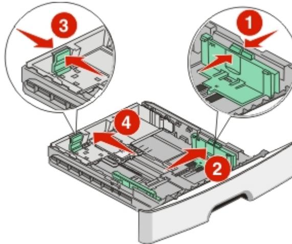
If you are loading a longer size of paper like A4 or legal, squeeze the length guide tab and slide the length guide backwards to
