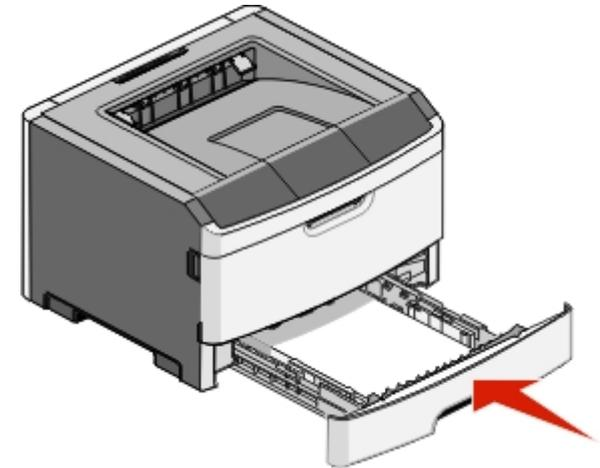
**8** If a different type of paper was loaded than the type previously loaded in the tray, change the Paper Type setting for the tray from the printer control panel. For more information, see "Setting the Paper Size and Paper Type" on page 5.
