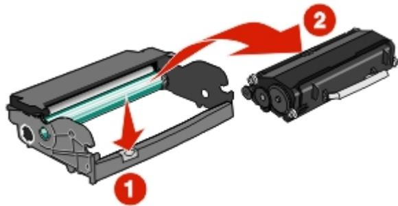
4 Unpack the new photoconductor kit. Be careful not to touch the photoconductor drum.
