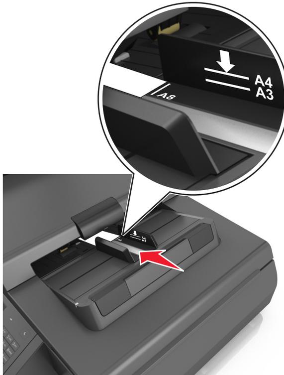
**Note:** Make sure the last edge of the business card is aligned with the A8 mark on the ADF guide.
