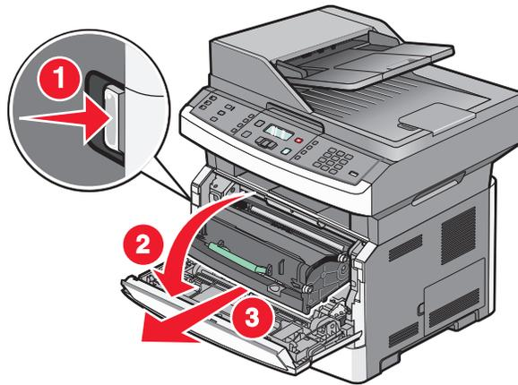
2 Lift the flap in front of the printer, and then remove any jammed sheets.
