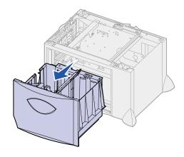
2 Squeeze the side guide lever, lift the guide, and place it into the appropriate slot for the size paper you are loading.
