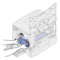
**c** Slide the image transfer unit out and place it on a clean, flat surface.
