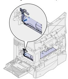
**7** Return the multipurpose feeder to its working position.
