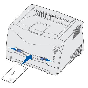
Warning: Do not force the print media into the feeder. Forcing the media causes jams.
