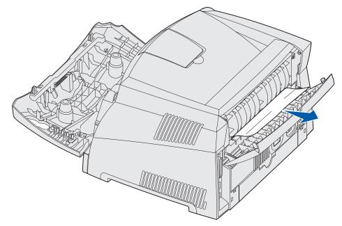
6 After you have cleared the jams, reinstall the print cartridge assembly, make sure all printer covers and trays are closed, and then press **Continue**  $\diamondsuit$  to resume printing.
