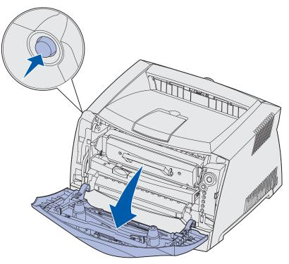
**2** Pull the print cartridge assembly out of the printer by pulling on the toner cartridge handle.
