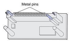
**3** Holding the card by its sides, align the pins on the card with the holes on the system board.
