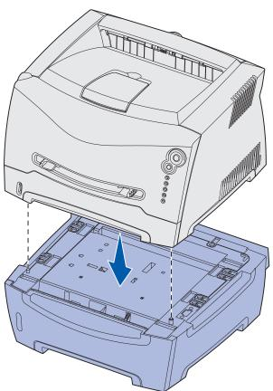
4 See How to get the printer driver to recognize installed options.
