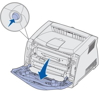
**3** Remove the print cartridge assembly out of the printer by pulling on the toner cartridge handle.
