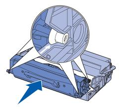
6 Install the print cartridge assembly into the printer by aligning the green arrows on the guides of the print cartridge assembly with the green arrows on the tracks in the printer and pushing the print cartridge assembly in as far as it will go.
