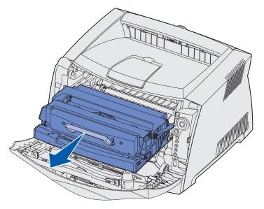
**Warning:** Do not leave the print cartridge assembly exposed to direct light for an extended period of time. Extended light exposure can cause print quality problems.
