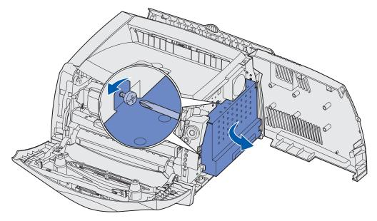
**5** Remove the metal plate by rotating it towards the front and to the right.
