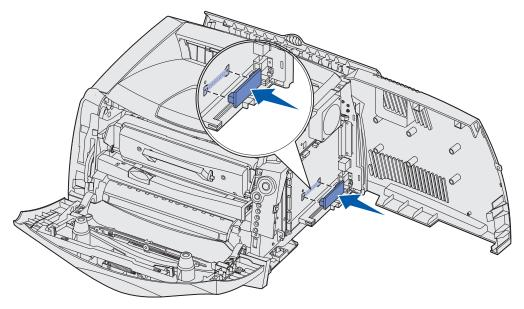
The entire length of the connector on the flash card must touch and be flush against the system board.
