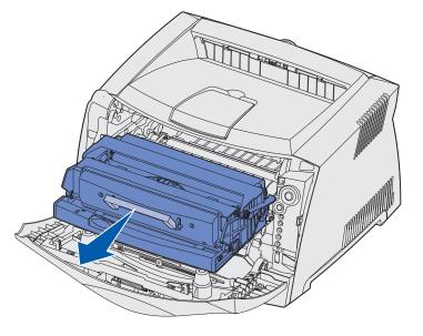
Note: Do not press the button on the print cartridge assembly.
