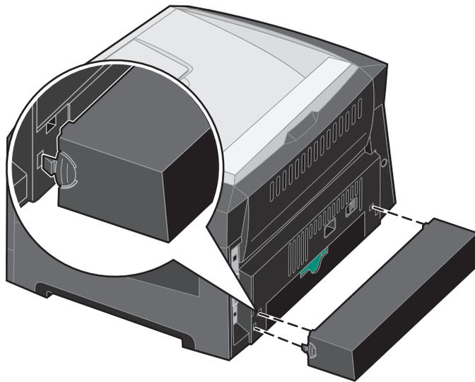
Attach the dust cover (if available) to the back of the printer by aligning the tabs on the cover to the holes on the printer, then *snap* the cover into place.
