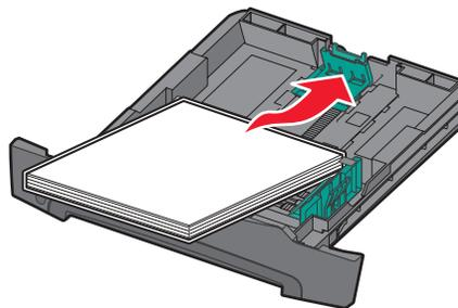
**Note:** Load letterhead paper with the design side facing down. The top edge of the sheet with the logo should be placed at the front of the tray.
